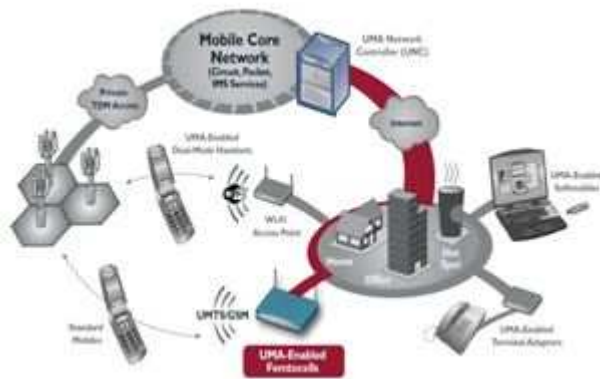
Figure 6: UMA the 3GPP standard for convergence provides high performance mobile coverage at home.
